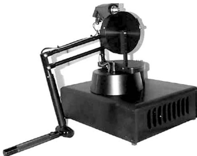
Fig. 1. Haptic device “Phantom 1.5/6DOF” by SensAble Technologies. The translational range of motion and force-feedback is 7.5 in.  $\times$  10.5 in.  $\times$  15 in., approximating the range of motion of the forearm. Torque feedback is provided through a powered gimbal. The rotational range of motion is 335° in the yaw and roll directions, and 260° in the pitch direction.
