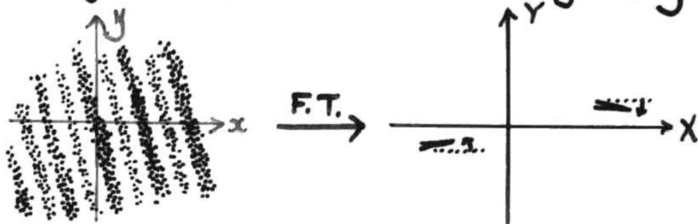
►  $\text{F.T.}[\text{F.T.}(\text{structure})] = \text{structure, rotated } 180^\circ$  Applies only to 2-D objects
